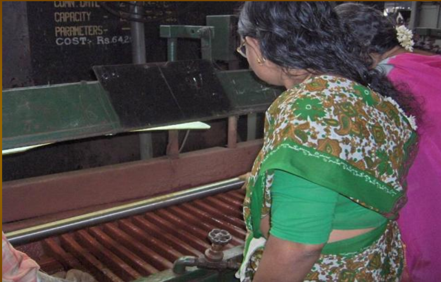
MAGNETIC PARTICLE INSPECTION OF SPRING BARS
